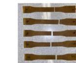
Thick SW/HW/CYCOM coupons after testing
